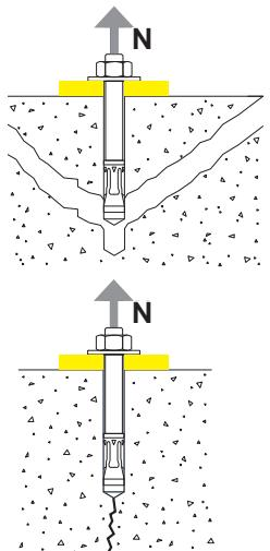
**WEDGE ANCHORS - ETA Approved (38AG)****Coefficients of influence**Influence of concrete strength resistance in pull-out failure  $\Psi_c$
